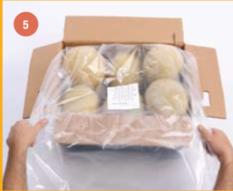
Pull the edges of the bag toward yourself in an orderly fashion (membranes should be on top of produce and free of wrinkles (as shown).
