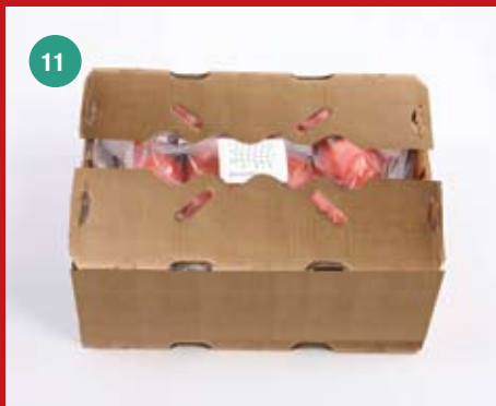
11 Apply case lid. Note: if the box has a solid lid, please cut a hole just above the membrane for atmosphere transfer.
